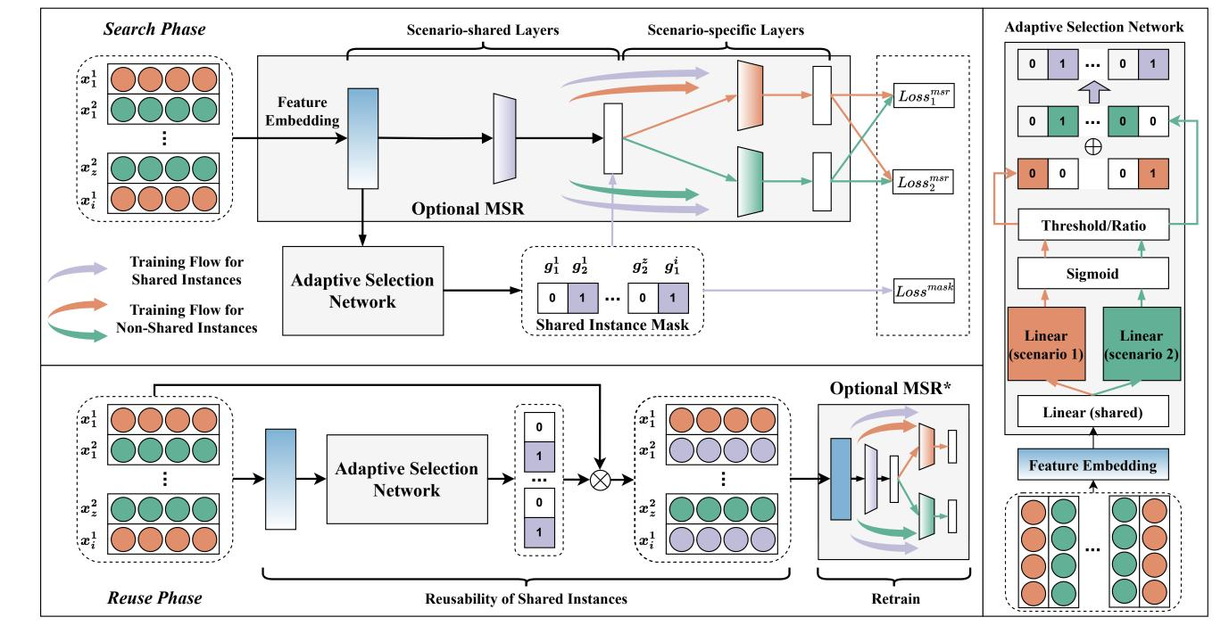
The SSIM framework includes two phases: search and retrain, and two key components: the backbone MSR model and the adaptive selection network.
